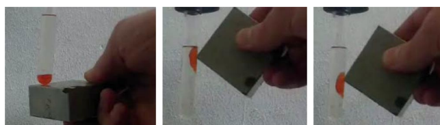
Figure 6. Response of the ionic liquid [\text{C}_6\text{mim}]_3[\text{Dy}(\text{SCN})_6(\text{H}_2\text{O})_2] to a neodymium magnet.
